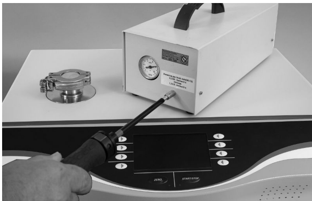
Fig. 12: Sniff test on an external calibration leak
