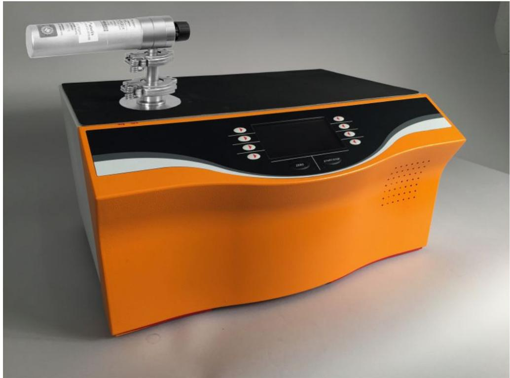
Fig. 15: Checking an external calibration leak
