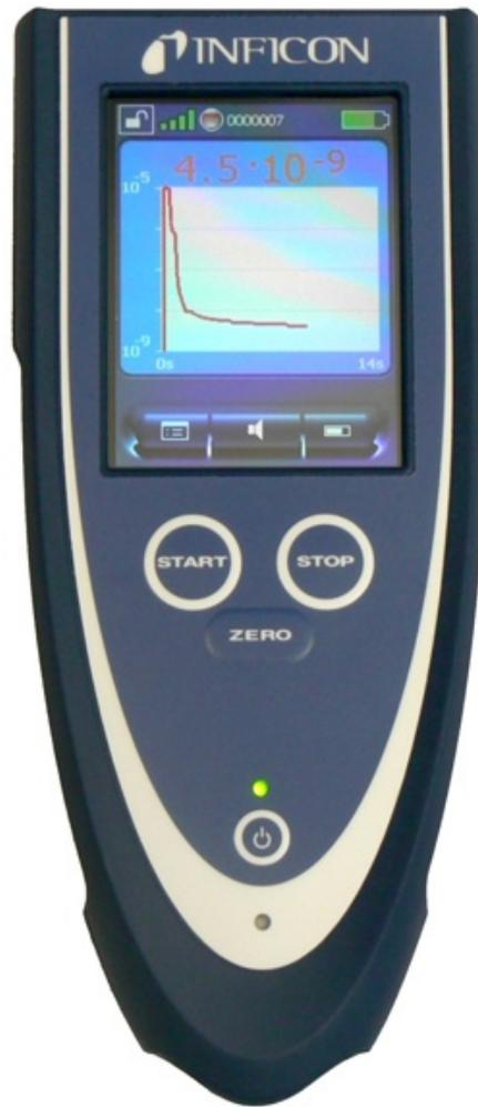
1. POWER button – Switches the RC1000 WL remote control on and off.
